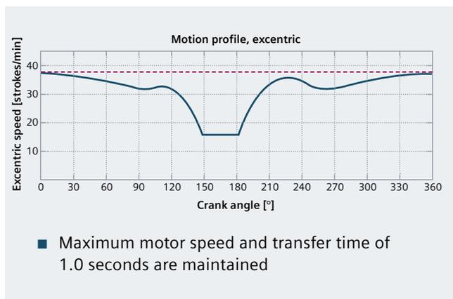
This particular press achieves a productivity of 30 strokes/minute with a press force of 2000 tons at 10 mm before BDC and 550 kJ forming work per stroke.
