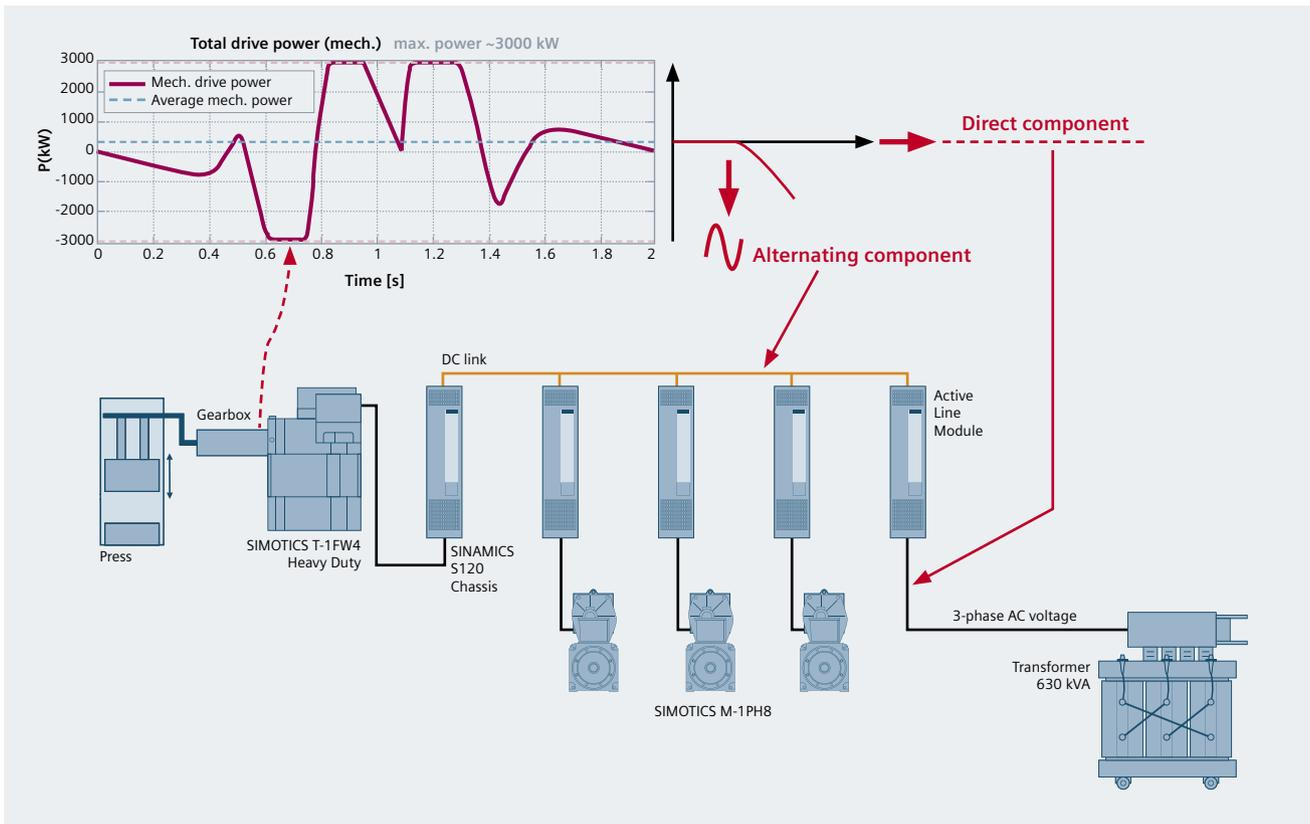
For the “full-size” energy management system, energy storage devices buffer the energy that is otherwise fed back into the line supply. As a consequence, the rms value of the infeed power is the same as the average value, thus preventing energy from being fed back into the line supply.
