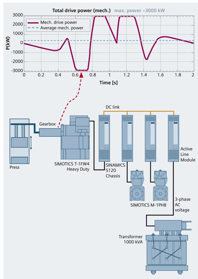
This means that the peak load is significantly higher than for the “full-size” energy management – and it fluctuates between a positive and negative load, between infeed and regenerative feedback. The supply transformer must also be correspondingly larger; and in this particular case, it must have a minimum 1000 kVA rating.
