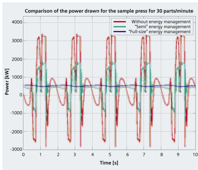
An almost constant infeed power and exclusively a positive power demand are only achieved with the “full-size” energy management system. For the other versions, the power drawn fluctuates significantly – and the regenerative feedback of electric power into the line supply, with all of its associated disadvantages.
