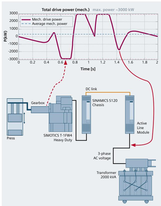
In this case, the infeed unit must cover a peak power of over 3000 kW, the upstream transformer must be able to handle these load peaks, and the significant load fluctuations directly impact the line supply. A transformer with a minimum rated power of 2000 kVA is required.
