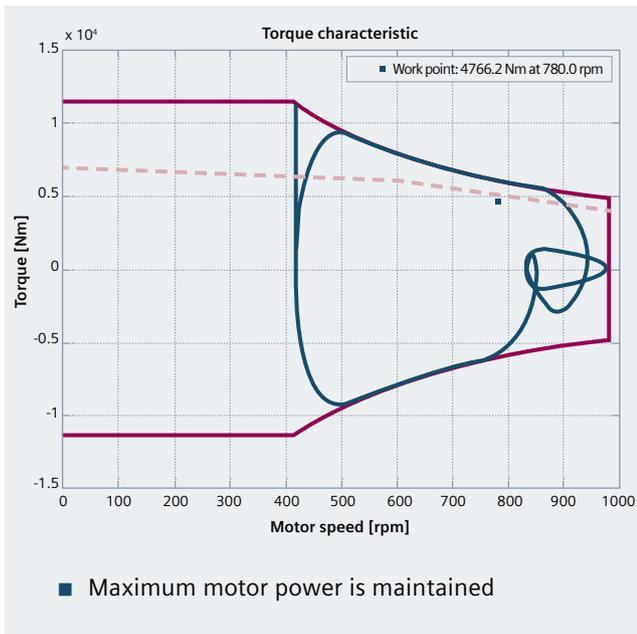
Siemens has integrated the new calculation technique into its SIMOTION motion control system: The OACAMGEN block automatically generates motion curves, which for the specified stroke rate, comply with all of the mechanical and electrical constraints of the overall system. As a consequence, the company operating the press has the maximum degree of flexibility. He can very simply adapt press motion to the die, material and part to be produced.
