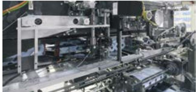
SINAMICS S120 and about 15 servo axes. This palletizer can be supplied with products in two ways and brings the individual packages into an optimized position on the pallets. A foil stretcher completes the line.
